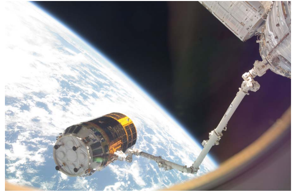
Figure 1: Capture of HTV by SSRMS ©JAXA
