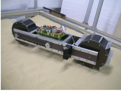
Figure 1. Two-wheeled rover.
