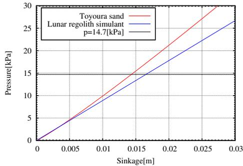
Figure 7. Pressure-sinkage relationship for Toyoura sand and lunar regolith simulant (for fixed  $l$  of 2.0 cm).
