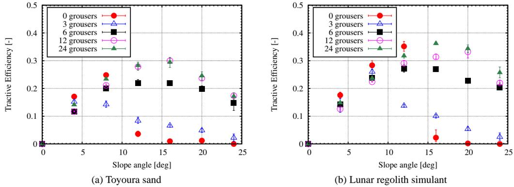
Figure 4. Slope angle versus tractive efficiency (for different numbers of grousers).
