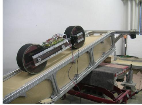
Figure 2. Slope-climbing test; the two-wheeled rover travels in a sandbox covered with Toyoura sand.
