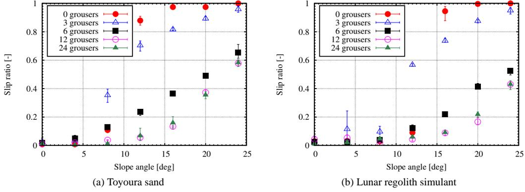
Figure 3. Slope angle versus slip ratio (for different numbers of grousers).
