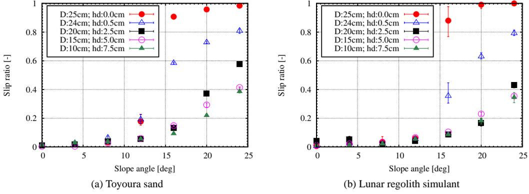
Figure 5. Slope angle versus slip ratio (for different grouser heights).
