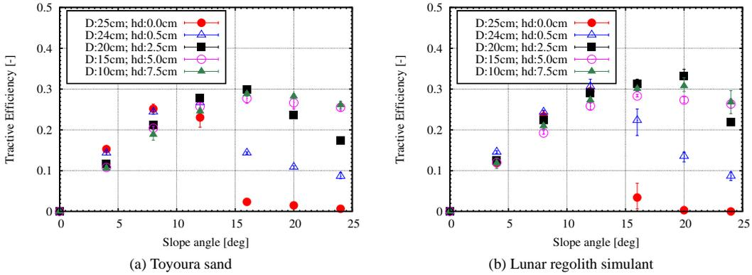
Figure 6. Slope angle versus tractive efficiency (for different grouser heights).
